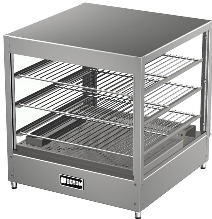
**Food Warmer/Display Case, Countertop, Three Shelf Interior Rack, Capacity (3) 18" Pizzas, Inside Water Pan for Humidity, Adjustable Heat Control, Tempered Glass Front, Sides & Door, Stainless Steel Construction, 120V/60/1P/8.2A**
