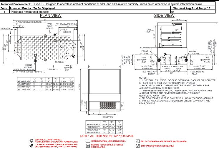
**Model Technical Specifications** Conv. Para. Rack Rack Amps **IaboM** 1 1" 1 2" **System Circuit Volts** Phs Fred Watts Wires **NEMA Plug** SST **BTUH** NR3647RSSV 35.75 Remote(Type II) 110-120 2+G Leads Single 20.00 263 N/A 60 1.05 Circuit #1 Self-Contained Circuit #1 110-120 60 16.00 1,18 2+G 5-20P or L5-20F N/A N/A NR4847RSSV 1.56 347
