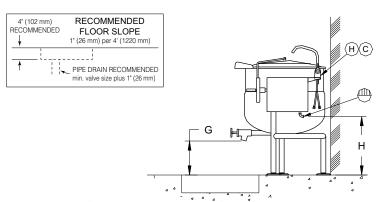
UNIT SHOWN WITH OPTIONAL 2" TANGENT DRAW-OFF VALVE, SPRING ASSIST COVER, HOT AND COLD WATER FAUCED AND STEAM CONTROL KIT.
