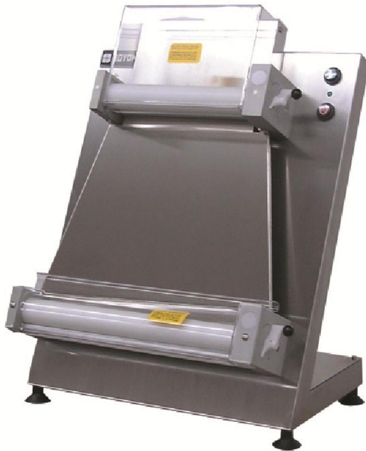
**Dough Sheeter, Countertop, Two (2) Sets of Rollers, Sheets up to 18" Wide, Up to 600 Pieces Per Hour, Teflon Rollers, Adjustable Roller Gap, Stainless Steel Scraper, Stainless Steel Construction, 1/2 HP Motor, cETLus, ETL-Sanitation**
