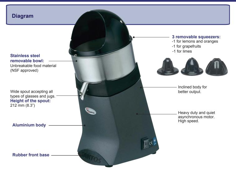
The citrus juice #52 is the perfect appliance to squeeze any kind of citrus thanks to the 3 removable squeezers (cones) delivered with the juicer. It is equipped with powerful and reliable commercial motor. You will easily extract from 20 to 40 liters per hour (5 to 10 gallons).
