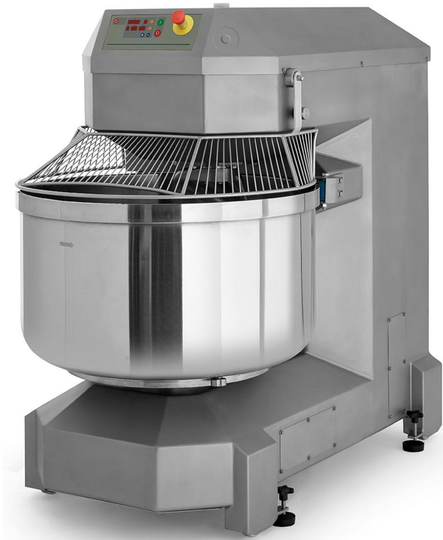
**Spiral Mixer, 350 Lb. Dough Capacity, 2 Speeds, Programmable Digital Control, Stationary Stainless Steel Bowl, Safety Guard & Dough Hook, Cast Iron Frame with Enamel Coated Steel Finish, 10 & 2 HP, 208-240/60/3P/32A, NEMA 15-30P**
