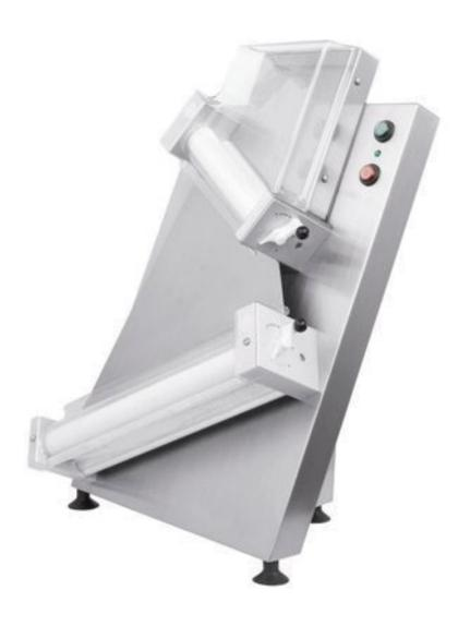
Dough Sheeter, Countertop, Two (2) Sets of Rollers, Sheets up to 18" Wide, Up to 600 Pieces Per Hour, Teflon Rollers, Adjustable Roller Gap, Stainless Steel Scraper, Stainless Steel Construction, 1/2 HP Motor, cETLus, ETL-Sanitation
