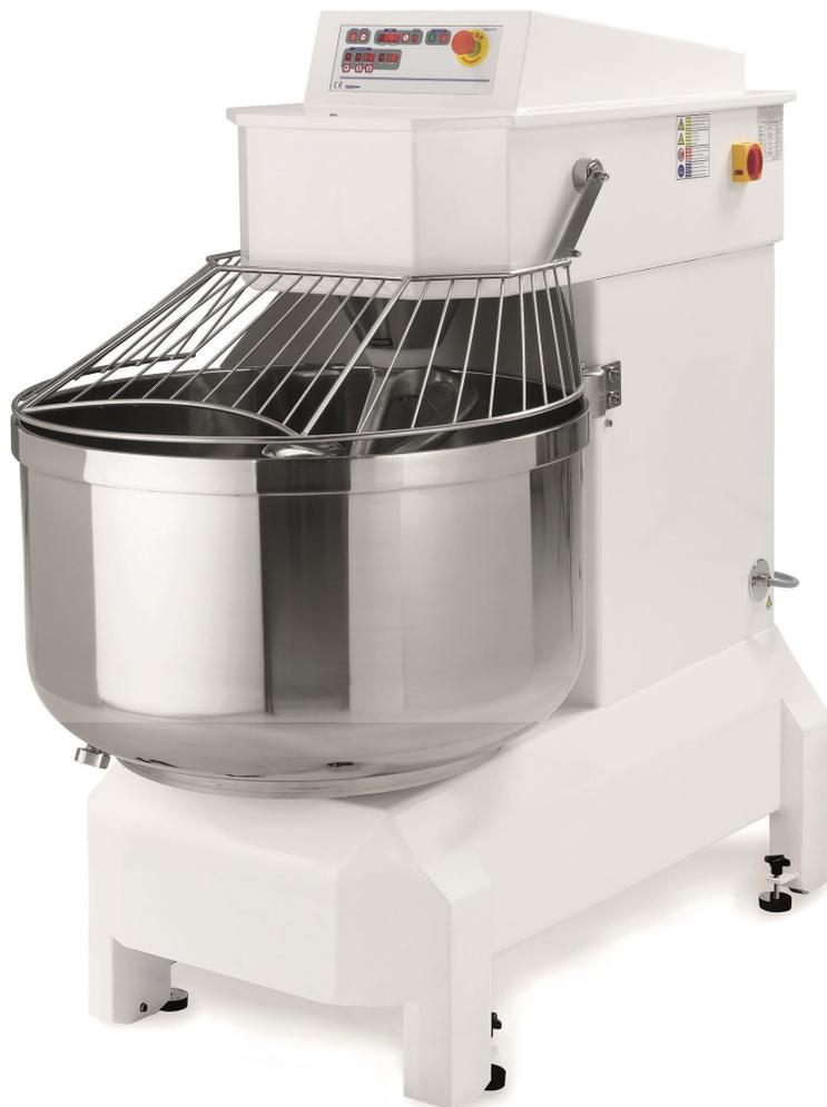
**Spiral Mixer, 280 Lb. Dough Capacity, 2 Speeds, Programmable Digital Control, Stationary Stainless Steel Bowl, Safety Guard & Dough Hook, Cast Iron Frame with Enamel Coated Steel Finish, 10 & 2 HP, 208-240/60/3P/32A, NEMA 15-30P**
