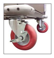
**HEAVY-DUTY PERFORMA CASTERS...** 5" diameter industrial grade casters with non-marking red rubber cushioned tread. Rust resistant Delrin bearings with all axles and raceways equipped with Zerk grease fittings. Long lasting and easy rolling, yet durable enough to withstand rigorous cart wash programs. Two fixed and two swivel casters with brakes for easy maneuvering.
