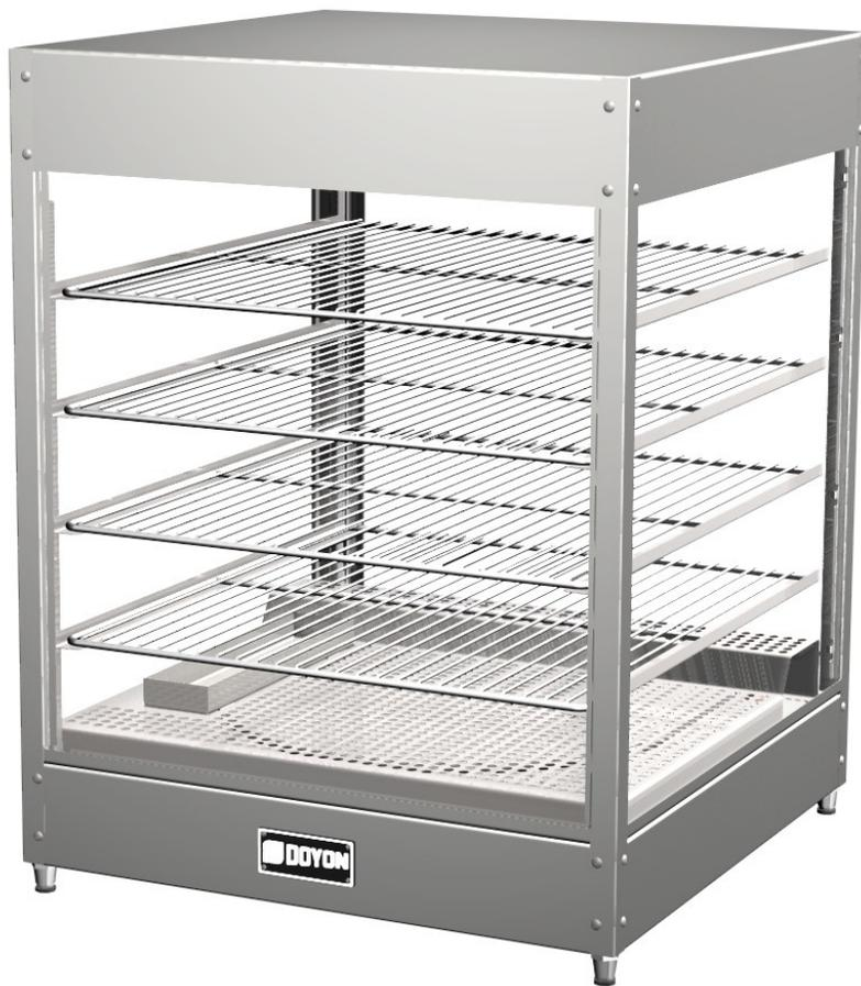
Food Warmer/Display Case, Countertop, Four Shelf Interior Rack, Capacity (4) 18" Pizzas, Inside Water Pan for Humidity, Adjustable Heat Control, Tempered Glass Front, Sides & Door, Stainless Steel Construction, No Top or Logo 120V/60/1P/8.2A
