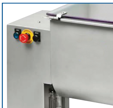
Emergency switch and safety microswitch
